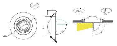
Through the unique structural design, it can be rotated 360° and retracted by 50°, which is convenient for irradiation, and the CRI can be selected as 80/90. The room temperature is optional (2700K/3000K/4000K/5000K), which increases the illumination range of the lamp and is more convenient to use.
