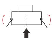
2. Put up spring dump before installing the downlight.
