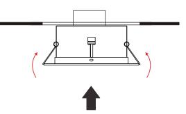
3. Insert the LED downlight to the hole like the picture schows.
