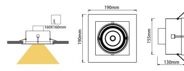
The LED recessed spots are presented in a simple design. The built-in spots are pleasantly modern and discreet. Recessed ceiling spotlights are light sources that can be used universally and can be installed in the different retail shop and large shopping mall.
