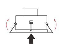
2. Put up spring dump before installing the downlight.
