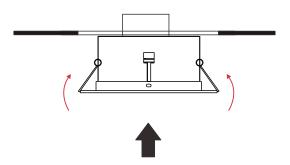
3. Insert the LED downlight to the hole like the picture schows.
