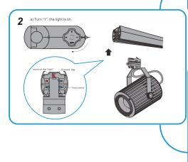
Step3: After fix the track light on the track system, then turn the switch make the lamp light on. Choose '1' or '2' or '3', and make the lamp 'on' and 'off'.
