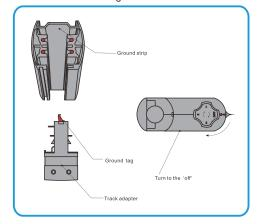
Step2: Attach the track light in the track system directy. Then turn the button fix the track light in the track system.
