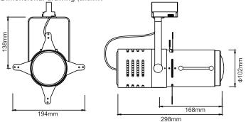
The gobo projector with specially designed lens to gain soft and even light effect from center to edge.
