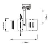
The gobo projector with specially designed lens to gain soft and even light effect from center to edge.
